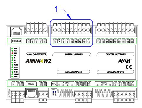
Fig. 5 - Inputs DI0.0 to DI0.7 connector location
