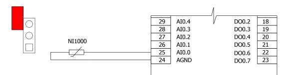
Fig. 22 - Connecting Ni1000 sensor
