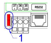
Fig. 29 - Connected jumpers on end station
