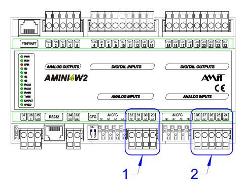
Fig. 12 - Inputs AI0.0 to AI0.7 connectors location
