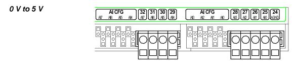
Fig. 14 - Setting configuration jumpers for range 0 V to 5 V
