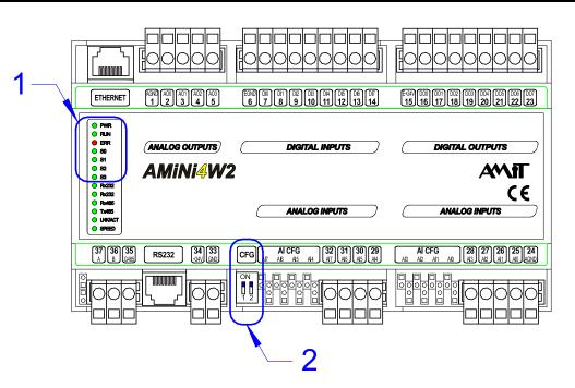
Fig. 33 - DIP switch and status indicator locations
