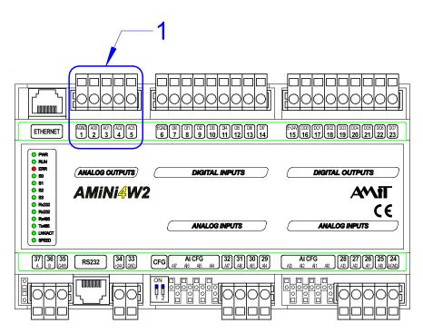
Fig. 23 - Outputs AO0.0 to AO0.3 connector location
