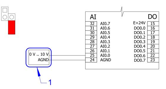
Fig. 20 - Connecting voltage sensor 0 V to 10 V
