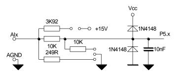
Fig. 13 - Wiring scheme of analogue input single channel
