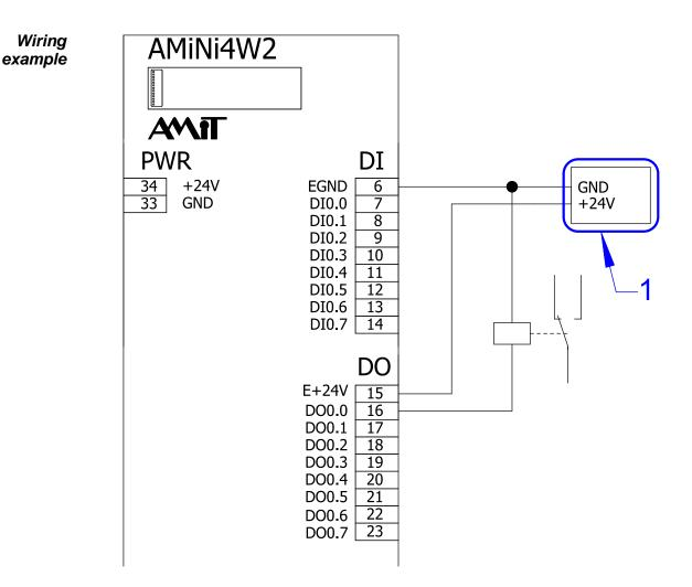
Fig. 11 - Operating the power contactor by semiconductor output
