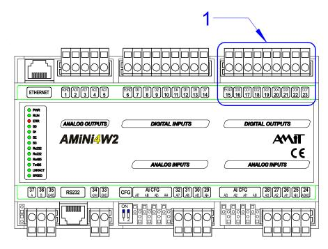
Fig. 10 - Outputs DO0.0 to DO0.7 connector location
