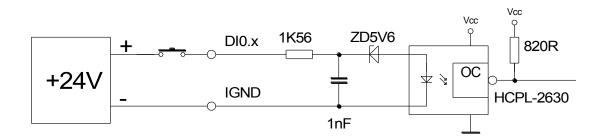
Fig. 6 - Wiring scheme of single digital input channel
