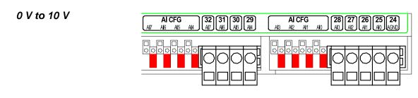
Fig. 15 - Setting configuration jumpers for 0 V to 10 V range, digital input 24 V
