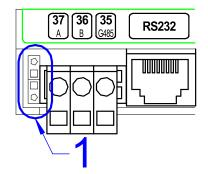
Fig. 30 - Disconnected jumpers on end station
