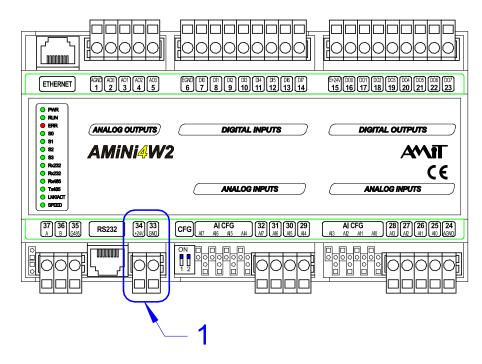
Fig. 3 - Power supply connector location
