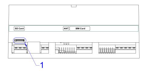
Fig. 32 - Micro SD card slot location
