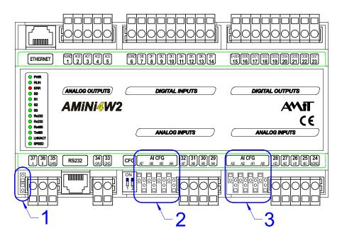
Fig. 34 - Configuration jumpers location
